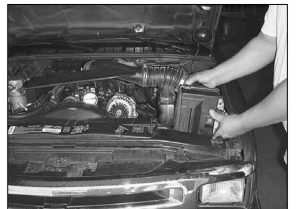
6. Remove the complete air intake assembly from the engine compartment.
