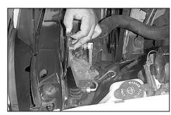
9. Pull the release tab and slide the retainer bracket upward to remove it from the radiator core
