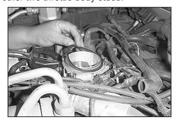
15. Install the gasket onto the throttle body flange.
