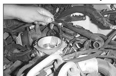
10. Using a 7/32" socket, loosen and remove the factory stand off from the throttle body.
