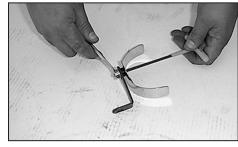
23. Assemble the L bracket and saddle bracket using the hardware provided.
