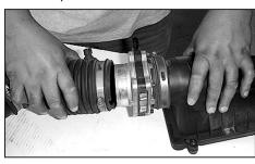
25. Remove the mass air sensor from the stock intake tube and air box top.
