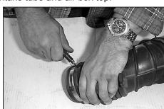
26. Remove the air temp. sensor from the stock intake tube and air box top.
