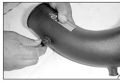
28. Install the air temp. sensor into the grommet.
