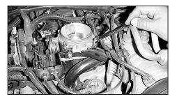
13. Install the short coupling nut onto the throttle body stud mentioned in the previous step.
