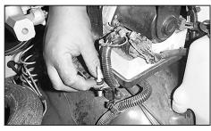
20. Install the 5/8" OD grommet and a flat washer over the original air box mounting stud.
