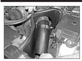
38. Install the secondary intake tube into the silicone hose and secure with provided hose clamp.
