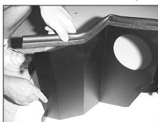
36. Install trim seal onto the heat shield. NOTE: Some cutting and trimming may be necessary for best fit.
