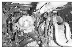
12. Remove the nut that retains the throttle cable bracket.
