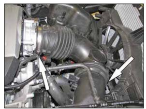
6. Loosen the hose clamps that secure the factory intake tube to the throttle body and air filter housing and then remove the factory intake tube from the vehicle.
