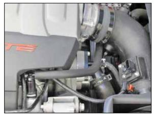
31. Reinstall the 90° quick disconnect fitting onto the valve cover port and then connect the open end of the hose to the fitting installed into the K&N<sup>®</sup> intake tube.
