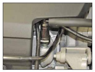
4A. On vehicles equipped with a "Wet Sump" oiling system, disconnect the crank case vent hose from the passenger side valve cover port and remove the hose from the vehicle.
