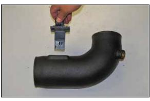
23. Install the mass air sensor assembly into the K&N<sup>®</sup> intake tube and secure with provided hardware.
