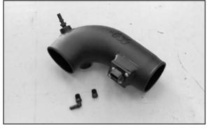
24. Install the provided vent fittings into the into the K&N $^{\mbox{\tiny B}}$  intake tube as shown.
