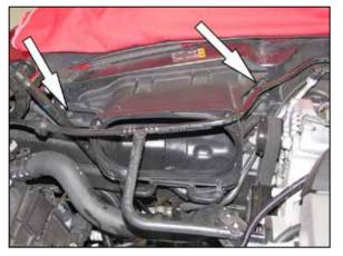
8. Remove the two bolts that secure the air filter housing to the inner fender then unhook the housing from the mounting stud and remove the housing from the vehicle. 12. Using a razor knife, cut the plastic hose at the TEE fitting where shown. Separate the plastic hose from the TEE fitting.
