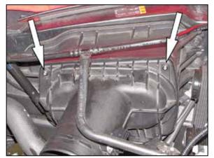
7. Loosen the two TORX fasteners securing the
