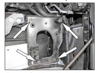
7. Remove the four bolts securing the air box mounting tray and then remove the tray from the vehicle.
