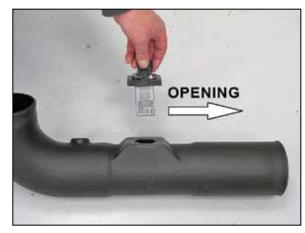
18. Install the mass air sensor assembly into the K&N intake tube and secure with the provided hardware.
