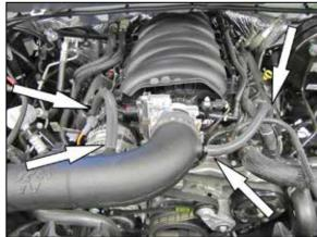
21. Connect the provided crank case vent hoses to the ports on the valve covers and then connect the open ends to the fittings installed into the K&N® intake tube.
