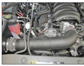
20. Install the K&N® intake tube into the hose at the filter adapter and then into the hose at the throttle body, adjust the tube for best fit and then secure with the provided hose clamps.
