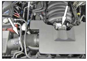
4. Loosen the two hose clamps securing the intake plenum to the factory air box and to the throttle
