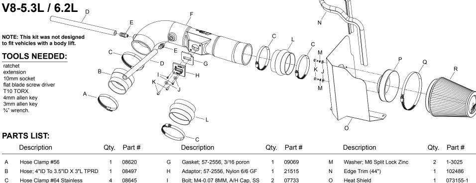
Hose Clamp #64 Stainless 08645 Bolt; M4-0.07 8MM, A/H Cap, SS 07733 Heat Shield 073155-1 Hose; 5/8" ID X 14"L Washer; 6MM Flat, SS 08269 Adapter; Universal, 6" Filter 084083 27300 Vent; STRT, 5/8 Barbed 1/4 NPT Bolt; M6 X 1.00 X 16MM, SS 07730 08911 Κ Q Hose Clamp #104 08697 Intake Tube 087268 Hose; 4"ID X 3"L Hump 08418 RF-1041
