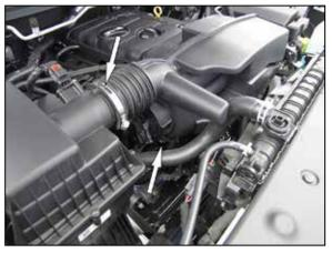
2. Loosen the hose clamps that secures the intake tube to the air filter housing and to the throttle body.
