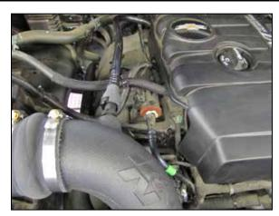
8. Install the provided coupler (08171) onto the K&N® intake tube and then install the intake tube into the coupler at the throttle body, align with the air filter housing and then position the coupler onto the housing. Adjust the tube for best fit and secure with the provided hose clamps. Reconnect the mass air sensor electrical connection. Connect the factory crank case vent line to the fitting installed into the K&N® intake tube.
