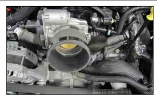
7. Install the provided straight coupler (084055) onto the throttle body and secure with the provided hose clamp.
