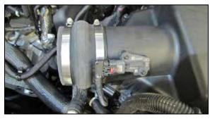
6. Install the provided hump coupler (08418) onto the air filter housing and secure with the provided hose clamp.
