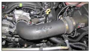
9. Install the K&N<sup>®</sup> intake tube into the coupler at the air filter housing and then into coupler on the throttle body, adjust the tube for best fit and then secure with the provided hose clamps.
