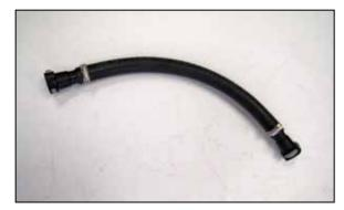
10. Assemble the crank case vent hose assembly as shown.
