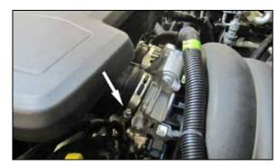
4. Loosen the hose clamp that secures the intake plenum to the throttle body. Rotate the plenum counter clockwise to unlatch it from the mounting bracket and then remove the plenum from the vehicle.
