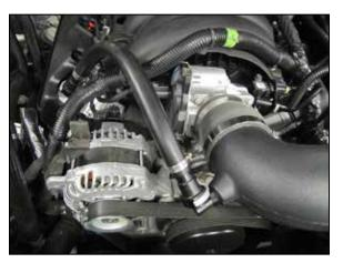
11. Connect the crankcase vent hose assembly to the fitting in the K&N $^{\odot}$  intake tube and to the valve cover port.
