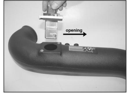
22. Install the mass air sensor assembly into the intake tube with the opening of the sensor pointing towards the air filter end of the tube as shown.
