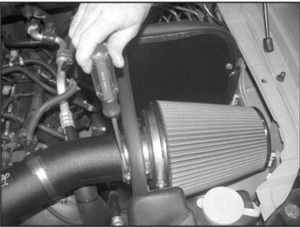
30. Install the K&N® air filter assembly onto the K&N® intake tube as shown; secure with the provided hose clamp.
