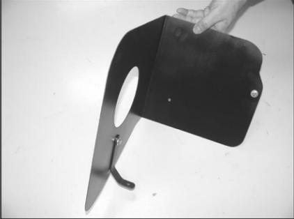
11. Install "L" bracket (07190) onto the heat shield as shown.
