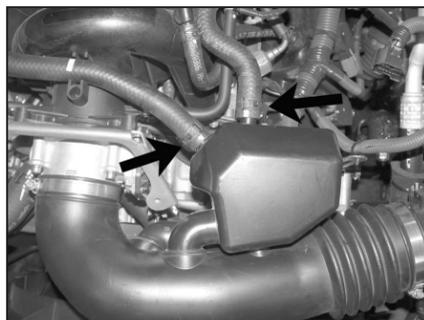
4. Remove the two vent lines from the air intake resonator as shown.
