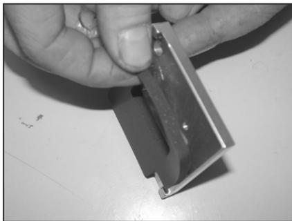
20. Apply the provided gasket to the mass air sensor adapter as shown; sticky side down.
