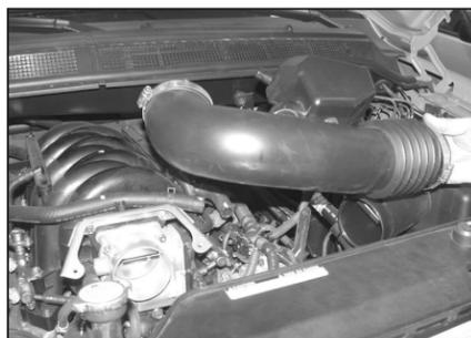
5. Loosen the hose clamps at the throttle body and air box, then remove the intake tube from the vehicle.
