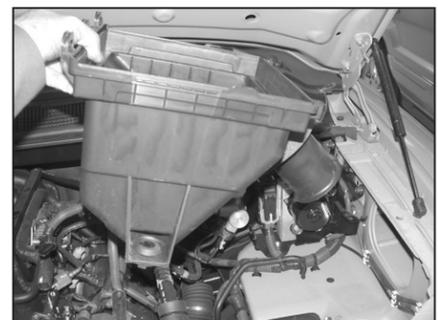
8. Pull firmly up on the air box to release it from the mounting studs, then remove the air box from the vehicle.
