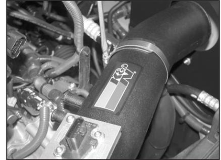
25. Secure the K&N® intake tube to the saddle bracket with the provided hose clamp. Also tighten the hose clamp at the throttle body.
