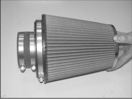
29. Install the filter adapter assembly into the K&N® air filter.
