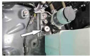
20. Install the provided 8mm rubber mounted stud into the resonator mounting location as shown.
