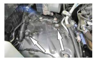
22. On 2005 through 2011 model year vehicles, install the two 6mm rubber mounted studs onto the inner fender as shown
