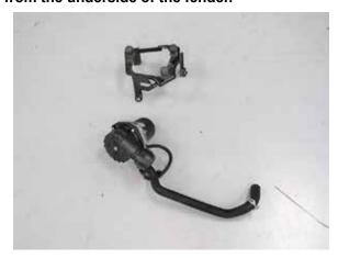
14. On vehicles equipped with secondary air injection, separate the secondary air pump mounting bracket from the pump motor.
