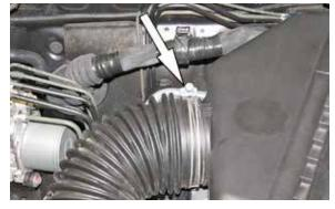
4. Loosen the hose clamp securing the intake hose to the air filter housing.
