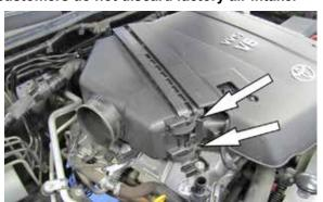
6. Release the two air box lid mounting clips and then remove the air box lid and factory air filter.
