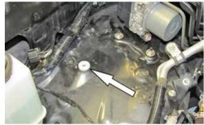
21. On 2012 and later model year vehicles, set the provided nylon spacer onto the inner fender heat shield mounting location as shown.
