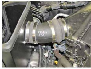
27. Install the K&N® intake tube into the hose at the filter adapter, align the hump hose with the air filter lid and then slide the hump hose onto the lid. Adjust the tube for proper fit and then secure with the provided hose clamps.
