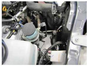
12. On vehicles equipped with secondary air injection, install the provided secondary air pump mounting bracket (083168) onto the power steering reservoir mount and secure with the factory retaining bolt from the previous step.
