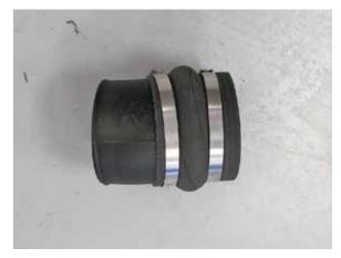
26. Install the provided hump coupler (087040) onto the K&N® intake tube all the way on as shown.
