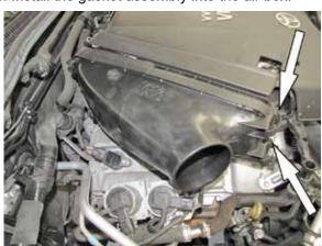
10. Install the K&N<sup>®</sup> air filter lid onto the air box and secure with the factory retaining clips.
