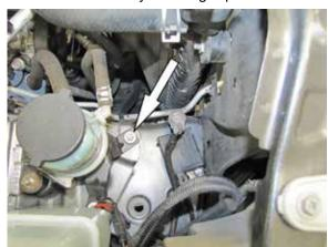
11. On vehicles equipped with secondary air injection, remove the power steering reservoir mounting bolt show.
