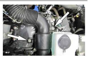
5. Remove the two bolts securing the resonator chamber to the inner fender and then remove the chamber and hose from the vehicle.
