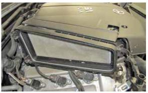
9. Install the gasket assembly into the air box.
