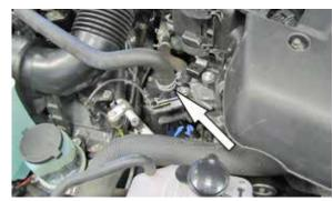
2. On Vehicles equipped with a secondary air pump, release the spring clamp securing the secondary air hose to the union on the engine and then disconnect the secondary air hose.
