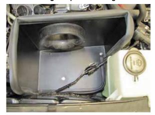
24. Reconnect the secondary air pump wiring harness connection.
