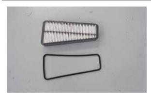
7. Remove the gasket from the factory air filter. NOTE: If the filter is not the factory filter with a non-removable gasket or if the gasket is damaged, it is recommended that a factory replacement air filter be purchased and the gasket removed and used.
