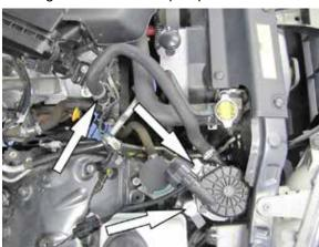
15. On vehicles equipped with secondary air injection, install the secondary air pump onto the brackets previously installed and secure with the provided hardware. Reconnect the secondary air hose to the fitting and secure with the factory spring clamp.
