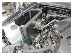
25. Install the provided coupling hose (08761) onto the filter adapter and secure with the provided hose
