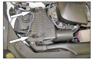
6. Install the  $K\&N^{\otimes}$  air filter and then resecure the clean side housing.
