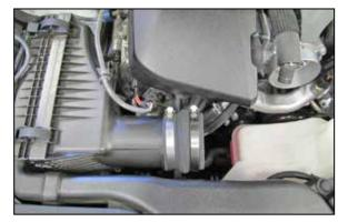
7. Install the coupling hose (08699) onto the air filter housing and secure with the provided hose
