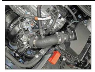
7. Install the K&N® intake tube into the coupler at the throttle body and then into the coupler on the air filter housing, adjust the tube for best fit and then secure with the provided hose clamps. Install the crank case vent hose onto the fitting and secure with the factory spring clamp.
