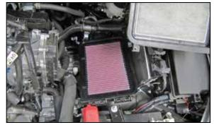
4. Release the clips that secure the upper air filter housing, lift up the housing and remove the factory air filter. Install the provided K&N® air filter and then reinstall the upper housing and secure with the factory retaining clips.
