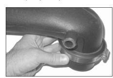
14. Fit the stepped rubber adaptor to the new plastic intake pipe using a #52 hose clamp supplied.
