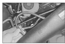
17. Fit the new grommet to the hole in the side of the intake pipe. Carefully insert the air temp sensor into the hole, reconnect the harness plug.
