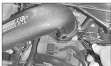
15. Attach the intake pipe/adaptor to the throttle
