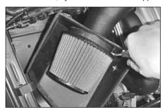
22. Fit the new Filtercharger to the intake pipe/filter adapter, ensure the filter sits flush with the heat shield, fully tighten the #72 hose clamp supplied.
