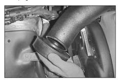
18. Fit the rubber filter adaptor to the end of the intake pipe.
