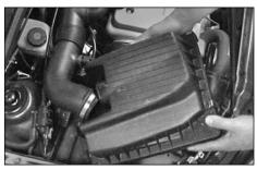
7. Slide the air box out of the lower mounting & carefully remove the complete air box from
