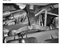
6. Remove the torx head screw securing the upper air box-mounting bracket.
