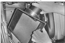
20. Fit the heat shield to the intake pipe assembly, ensure the rubber adapter lip sits up against the shield.
