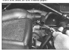
11. Unclip & remove the intake pipe from the throttle housing.
