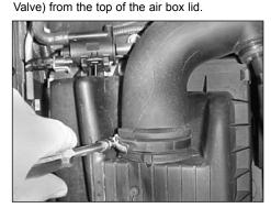
5. Unclip & remove the intake pipe from the air box lid.
