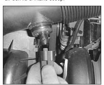
3. Unclip & remove the harness plug from the air temp sensor, carefully remove the sensor from the intake pipe.
