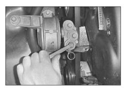
12. Remove the front bolt from the side engine
