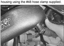
16. Fit the engine breather hose to the intake pipe using the original hose clamp.
