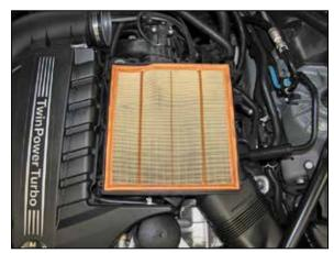
3. Loosen the six screws that secure the upper air filter housing to the lower housing, then remove the upper housing and factory air filter from the vehicle NOTE: K&N Engineering, Inc., recommends that customers do not discard factory air intake.
