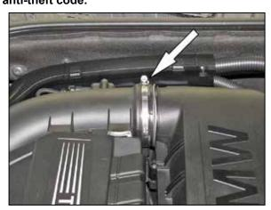
2. Loosen the hose clamp securing the upper air filter housing to the intake tube.
