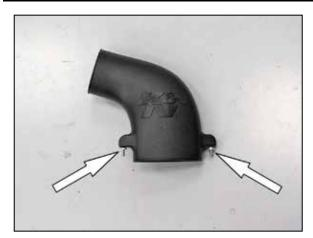
6. Install the two provided studs and spacers onto the  $K\&N^{\otimes}$  intake tube as shown.
