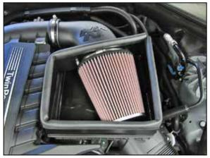
8. Install the K&N<sup>®</sup> air filter onto the intake tube and secure with the provided hose clamp.
