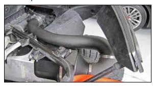
29. Install the K&N® fresh air intake tube assembly and 90° coupler hose (08502) to the fresh air tube mount and air filter housing, adjust for best fit and the secure with the provided hose clamps.
