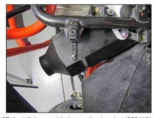
27. Install the provided mounting bracket (083110) as shown using the provided hardware. NOTE: The frame side of the bracket will be secured once the package tray is reinstalled.
