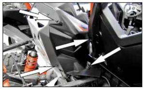
5. Remove the four bolts that secure the right side charger air cooler cover and then remove the cover
