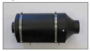
24. Secure the air filter housing to the bracket with the hose clamps as shown.
