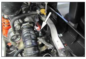
11. Partially remove the air filter assembly to gain access to the crank case vent hose connection to the intake tube. Cut the pinch clamp securing the crank case vent hose and then disconnect the hose from the intake tube and then completely remove the air filter system.
