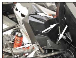
30. Reinstall the charge air cooler cover and secure with the factory bolts.
