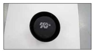
21. Install the K&N® air filter assembly into the housing and secure with the provided hardware.
