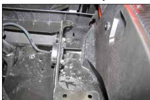
12. Remove the two bolts that secure the fresh air tube mount to the body and remove the mount. NOTE: The bolts are accessed from the underside. These bolts will be reused in the next step.
