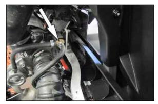
7. Cut the pinch clamp securing the waste gate valve vacuum hose and then disconnect the vacuum hose from the vacuum switch.
