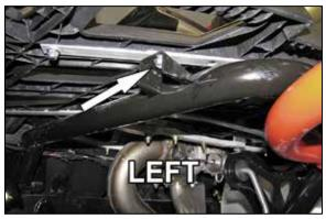
3. Remove the bolts that secure the package tray from the underside.
