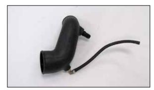
16. Install the waste gate hose and fitting along with the provided crank case vent hose fitting into the K&N® intake tube as shown.
