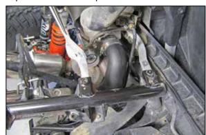
19. Install the K&N® intake tube into the coupler hose and secure with the provided hose clamp. Connect the waste gate vacuum hose to the vacuum switch and secure with the provided tie
