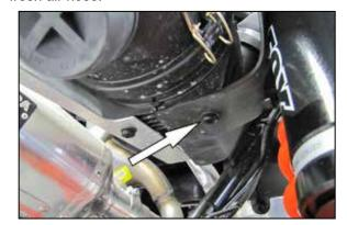
10. Remove the three bolts that secure the air filter assembly.
