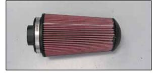
20. Install the provided filter adapter into the K&N® air filter and secure with the provided hose clamp.
