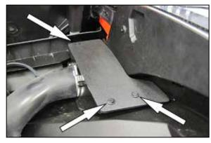
6. Remove the three push clips and then remove the fresh air dust cover.
