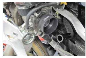
17. Install the provided coupler hose (08682) onto the turbo inlet and secure with the provided hose clamp.
