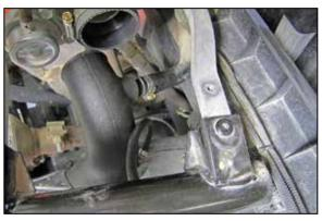
18. Connect the crank case vent hose to the fitting installed into the K&N<sup>®</sup> intake tube and secure with the provided hose clamp.
