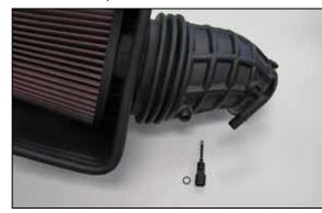
9. Remove the inlet air temperature sensor from the factory intake tube.
