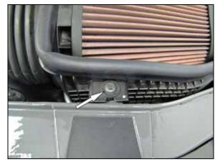
Remove the bolt that secures the air filter housing to the core support.
