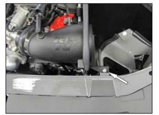
14. Secure the heat shield to the core support with the provided hardware then secure the intake tube with the provided hose clamp.
