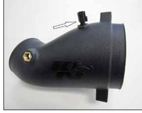
10. Install the provided grommet into the K&N® intake tube, then remove the o-ring from the inlet air temperature sensor and install the sensor into the grommet.
