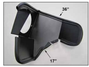
7. Install the edge trim onto the heat shield as shown.
