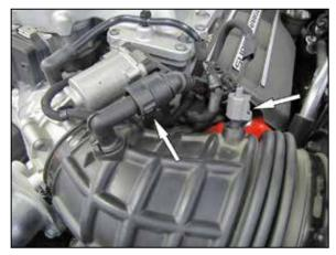
2. Disconnect the inlet air temperature sensor electrical connection and the crank case vent line from the factory intake tube.
