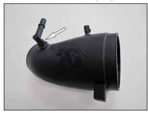
11. Install the provided 90° quick disconnect fitting into the K&N<sup>®</sup> intake tube as shown. NOTE: Plastic NPT fittings are easy to cross thread. Install the vent fitting "hand" tight, then turn it two complete turns with a wrench.
