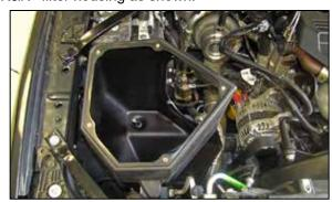
12. Install the K&N® filter housing into the vehicle so the mounting pins protrude through the grommets.
