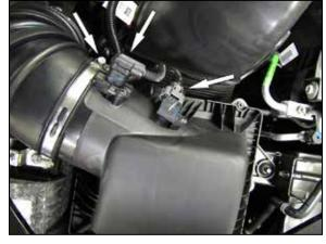
4. Loosen the hose clamp the secures the intake tube to the air filter housing and disconnect the electrical connections of the two air sensors.
