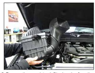
5. Remove the complete air filter housing from the vehicle as shown.
