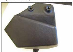
11. Remove the mounting grommets from the factory air filter housing and install them into the K&N® filter housing as shown.
