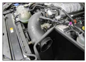
14. Install the K&N intake tube into the heat shield and then into the coupler, align for best fit and then secure with the provided hardware and hose clamp.
