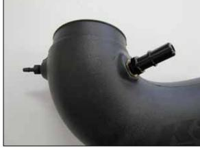
13. Install the provided vent fittings into the K&N intake tube as shown.
