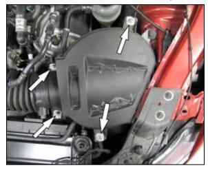
4. Remove the four bolts that secure the air filter lid and then remove the lid from the vehicle.
