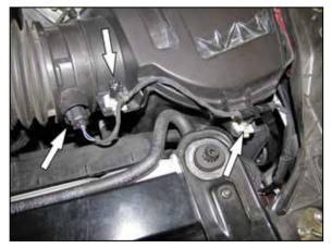
2. Disconnect the IAT sensor electrical connection and unhook the wiring harness from the air filter housing. 3. Disconnect the two vent lines attached to the factory intake tube. Loosen the hose clamp that secures the intake tube to the throttle body.
