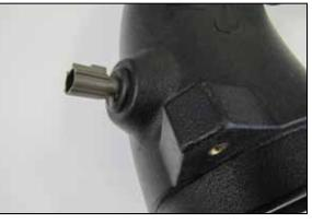
12. Remove the IAT sensor from the factory intake tube and install it into the K&N intake tube using the provided grommet.
