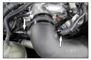
15. Connect the two factory vent lines to the fittings installed into the K&N intake tube.
