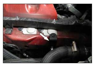
7. Secure the heat shield mounting bracket to the inner fender using the provided hardware.
