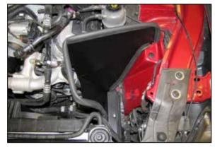
10. Install the heat shield into the vehicle and secure it to the inner fender and mounting bracket with the provided hardware.
