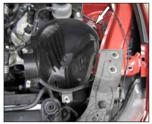
6. Remove the bolt that secures the factory air box to the inner fender and then remove it from the vehicle.
