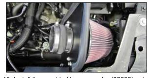
13. Install the provided hump coupler (08699) onto the filter adapter and secure with the provided hardware.
