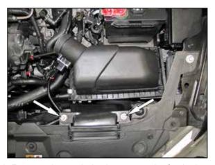
6. Remove the two bolts that secure the fresh air duct to the core support then lift up and remove the complete air filter housing from the vehicle.
