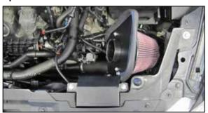
12. Install the heat shield assembly so the mounting studs insert into the air filter housing mounting grommets. Secure the fresh air duct with the hardware provided to the core support and the hardware installed into the heat shield.
