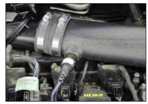
20. Connect the EVAP vent line to the quick disconnect fitting installed into the K&N® intake
