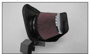
11. Install the K&N® air filter onto the filter adapter and secure with the provided hose clamp. NOTE: Drycharger® air filter wrap; part # 22-8049DK is available to purchase separately. To learn more about Drycharger® filter wraps or look up color availability please visit http://www.knfilters.com®.
