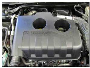
3. Lift the engine cover and remove it from the vehicle.
