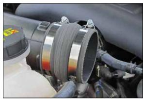
14. Install the provided coupler hose (087121) onto the passenger side turbo inlet hose and secure with the provided hose clamp.
