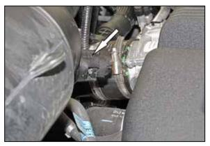
2. Disconnect the inlet air temperature sensor electrical connector and remove the tape around the harness connector.
