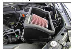
11. Install the heat shield/filter assembly onto the factory lower air filter housing and secure with the factory retaining clips.
