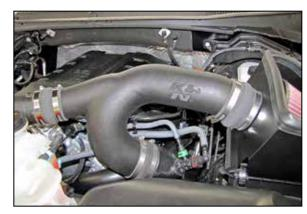
17. Install the K&N® intake tube into the couplers at the turbo inlet tubes and then into the coupler at the filter adapter, adjust the tubes for best fit and then secure with the provided hose clamps.
