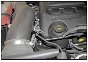
18. Reconnect the inlet air temperature sensor electrical connection.
