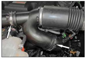
5. Loosen the two hose clamps that secure the factory intake tube to the turbo inlets, then remove the factory intake tube from the vehicle. NOTE: K&N Engineering, Inc., recommends that customers do not discard factory air intake.
