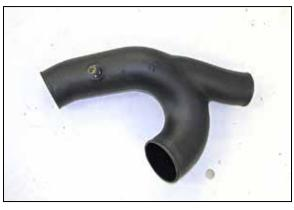
16. Install the provided grommet and inlet air temperature sensor into the K&N® intake tube as show.
