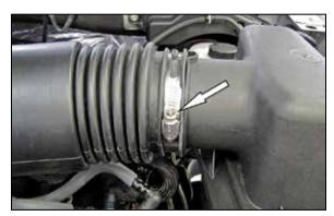
3. Loosen the hose clamp that secures the factory intake tube to the upper air filter housing.
