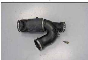
15. Remove the inlet temperature sensor from the factory intake tube.
