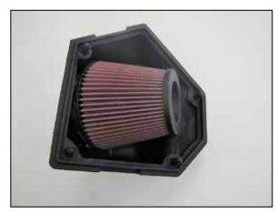
17. Install the filter assembly into the upper K&N<sup>®</sup> air filter housing and secure with the provided hardware
