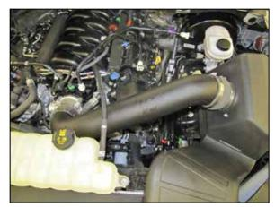
22. Install the K&N® intake tube into the couplers, adjust for best fit and then secure with the provided hose clamps.
