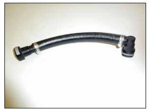
24. On vehicles that have the CCV hose connected to the valve cover between the second and third coil pack, assemble the provided CCV hose as shown.
