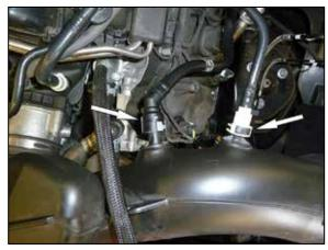
2. Depress the locking tabs and then disconnect the crank case vent and EVAP vent lines.
