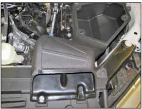
15. Install the two provided retaining clips to secure the fresh air scoop to the core support.
