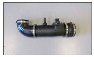
21. Install the provided angle hose #08629 and hump hose #08493 onto the K&N® intake tube but do not completely tighten at this time.
