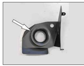
8. Install the filter adapter into the K&N® heat shield and secure with the provided hardware.
