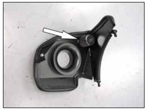
13. Install the quick connect adapter and crank case breather filter onto the heat shield as shown.
