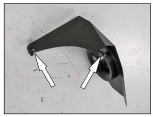
9. Install the two provided mounting studs onto the heat shield using the provided hardware.
