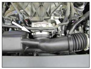
6. Loosen the hose clamp securing the intake tube to the throttle body. Disconnect the factory intake tube from the throttle body.
