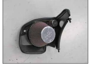
14. Install the K&N<sup>®</sup> air filter onto the filter adapter and secure with the provided hose clamp. NOTE: Drycharger<sup>®</sup> air filter wrap; part # 22-8049DK is available to purchase separately. To learn more about Drycharger® filter wraps or look up color availability please visit http://www.knfilters.com®.
