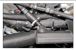
3. Release the locking tap and then disconnect the EVAP vent line quick disconnect fitting from the factory intake tube.
