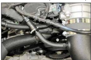
27. Connect the K&N® EVAP quick disconnect fitting into the factory fitting.
