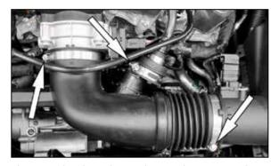
5. Loosen the three hose clamps that secure the intake tube and crank case vent tube then remove the intake tube from vehicle.
