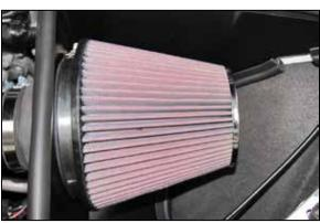
30. Install the K&N® air filter and secure with the provided hose clamp.
