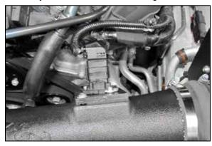
29. Reconnect the mass air sensor electrical connection.
