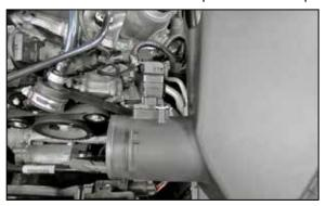
9. Disconnect the mass air sensor electrical connection.
