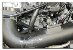
28. Install the provided crank case vent hose onto the factory vent hose and K&N® fitting.
