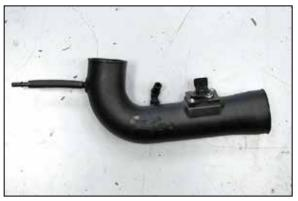
25. Install the 90° crank case vent fitting into the K&N® intake tube as shown.
