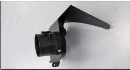
7. Install the K&N® mass air housing into the heat shield and secure with the provided hardware.
