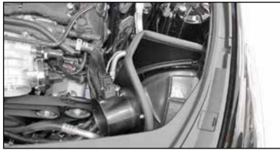
13. Install the heat shield assembly into the vehicle so that the mounting studs engage into the factory air filter housing mounting grommets.
