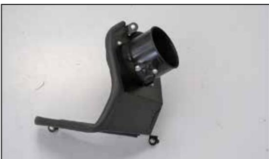
12. Install the mass air sensor into the K&N® air filter housing and secure with the provided hardware.
