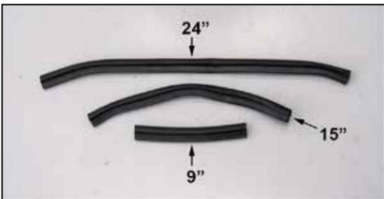
9. Cut the provided edge trim into three sections of 24", 15" and 9" as shown.
