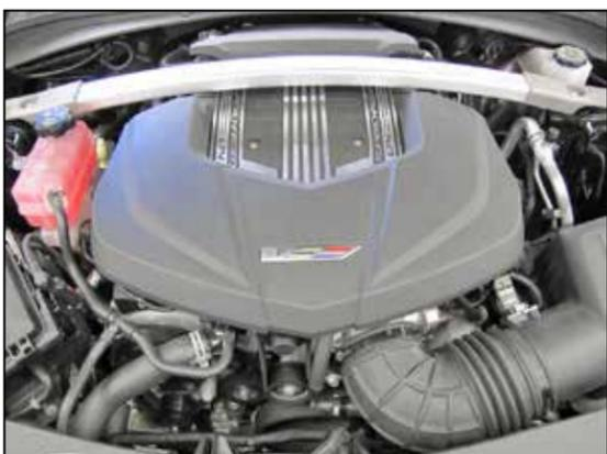
2. Lift the decorative engine cover and remove it from the engine.
