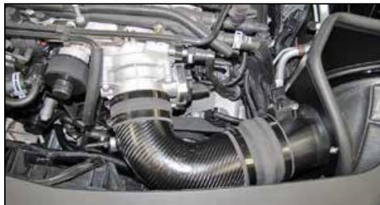
17. Install the intake tube assembly into the hump coupler and then into the coupler at the throttle body, adjust the tube for best fit and then secure with the provided hose clamps.
