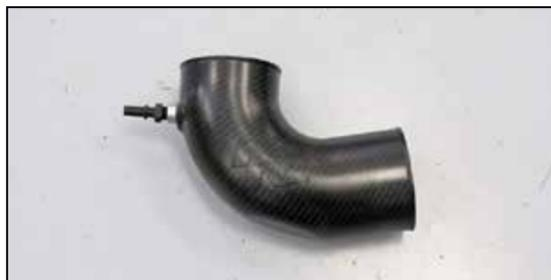
16. Install the provided NPT quick disconnect fitting into the K&N® intake tube.
