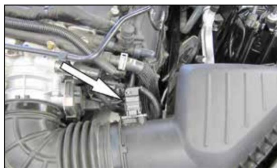
3. Disconnect the mass air sensor electrical connection.
