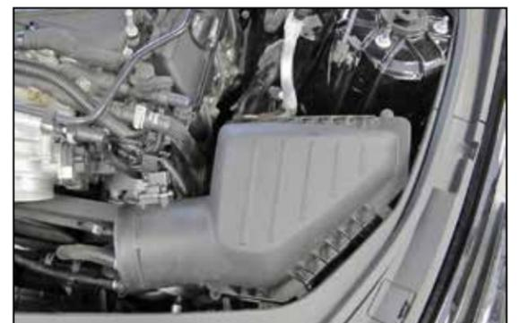
6. Lift the air filter housing assembly and remove it from the vehicle.
