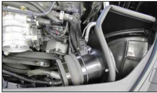
14. Install the provided hump coupler hose (084101) onto the mass air sensor housing and secure with the provided hose clamp.
