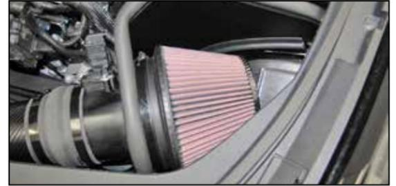
20. Install the K&N® air filter and secure with the provided hose clamp.
