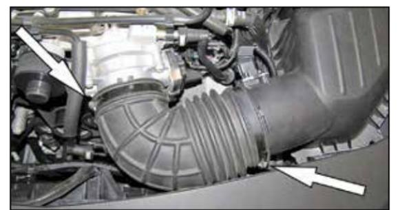
5. Loosen the hose clamps that secure the factory intake hose to the throttle body and air filter housing.
