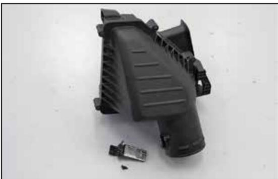
11. Remove the mass air sensor from the factory air filter housing.
