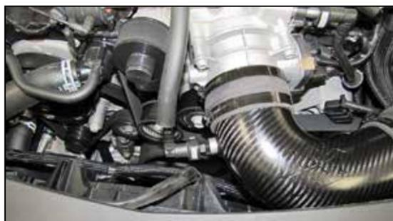
18. Connect the crank case vent fitting to the quick disconnect fitting installed into the K&N® intake tube.
