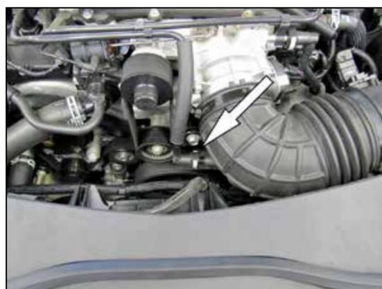
4. Disconnect the crank case vent quick disconnect fitting.
