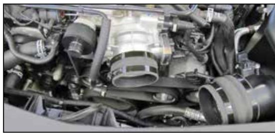
15. Install the provided coupler hose (08618) onto the throttle body and secure with the provided hose clamp.
