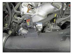
13. Reconnect the mass air sensor electrical connection and secure the red locking tab.
