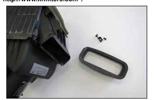
15. Remove the fresh air bellows from the factory air filter housing lid.
