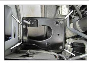
5. Remove the four bolts that secure air filter mounting tray and then remove the tray from the vehicle. Three of the factory bolts will be reused in a later step.
