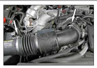
3. Loosen the two hose clamps securing the factory intake tube to the turbo inlet and air filter housing, then remove the factory intake tube from the vehicle.
