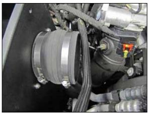
8. Install the provided hump coupler (08418) onto the filter adapter and secure with the provided hose clamp.
