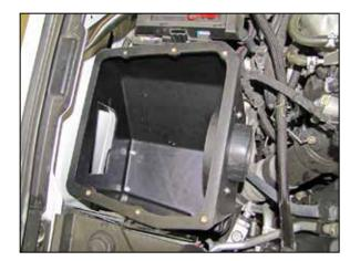
7. Install the K&N® air filter housing into the vehicle and secure it to the factory housing mounting plate fastener location with the hardware removed in step 5.
