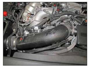
12. Install the K&N® intake tube assembly into the coupler at the filter adapter and then into the factory turbo inlet coupler. Adjust the tube for best fit and then secure with the hose clamps.
