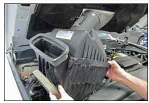
4. Lift up the air filter housing to release it from the mounting grommets and then remove the air filter housing from the vehicle.
