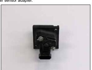
10. Remove the mass air sensor from the factory air filter housing and then install it into the K&N® adapter and secure with the provided hardware.
