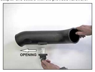
11. Install the sensor assembly into the K&N® intake tube and secure with the provided hardware. NOTE: Be sure to install the sensor in the correct direction, the opening in the sensor should be pointed towards the filter end of the tube.
