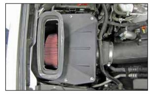
17. Install the K&N® air filter housing lid onto the filter housing and secure with the provided hardware.
