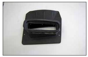
16. Install the bellows onto the K&N® air filter housing lid and secure with the factory retaining
