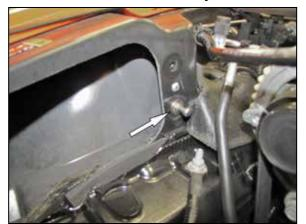
9. Remove the air filter housing mounting stud from the inner fender.
