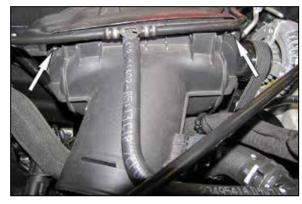
7. Loosen the two screws that secure the mass air sensor housing to the air filter housing and then remove the mass air sensor housing from the vehicle.
