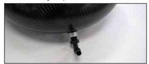
17. Install the provided crank case quick connect fitting into the K&N® intake tube as shown. **NOTE: Plastic NPT fittings are easy to cross** thread. Install the vent fitting "hand" tight, then turn it two complete turns with a wrench.
