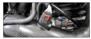
20. Using the provided extension harness, reconnect the mass air sensor electrical connection.
