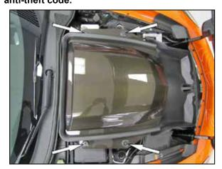
2. Loosen the four bolts that secure the super charger cover, remove the bolts and then remove the cover from the vehicle.
