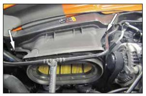
8. Remove the two bolts that secure the air filter housing to the inner fender and then remove the housing and air filter from the vehicle.
