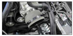
15. Install the provided coupler (08633) onto the throttle body and secure with the provided hose clamp.
