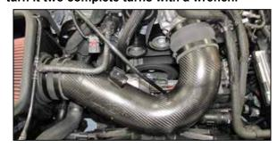
18. Install the K&N® intake tube into the coupler hose at the air filter and then into the coupler at the throttle body. Adjust the tube for best fit and then secure with the provided hose clamps.
