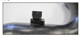
16. Remove the mass air sensor from the factory mass air sensor housing and install it into the K&N® intake tube using the provided hardware.
