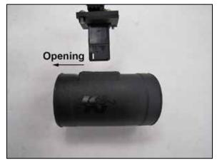
11. Remove the mass air sensor from the factory housing. Install the mass air sensor into the adapter provided and secure with the provided hardware. Install the provided gasket onto the adapter and then install the assembly into the K&N® intake tube and secure with the provided hardware. NOTE: Be sure to install the sensor assembly in the direction shown, the open end of the sensor is to be towards the air filter.
