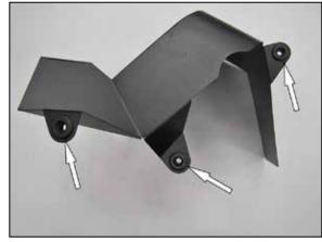
6. Remove the three mounting grommets from the factory air filter housing and install them into the K&N® heat shield as shown.
