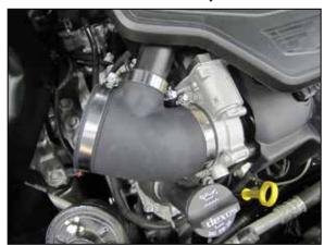
10. Install the provided coupler onto the throttle body and intake plenum. Secure with the provided hose clamps.
