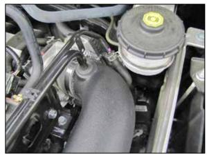
20. Install the crank case vent tube into the grommet installed into the  $K\&N^{\otimes}$  intake tube.
