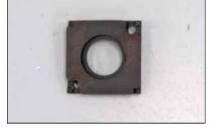
15. Install the provided gasket onto the K&N<sup>®</sup> mass air sensor adapter as shown.
