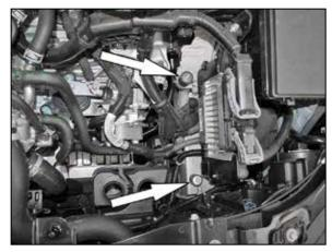
7. Install the two provided rubber mounted studs onto the air filter housing mounting locations as shown.
