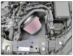
12. Install the K&N $^{\odot}$  air filter onto the filter adapter and secure with the provided hose clamp.
