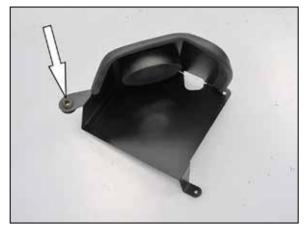
10. Remove the mounting grommet from the factory air filter housing and install it into the K&N<sup>®</sup> heat shield as shown.
