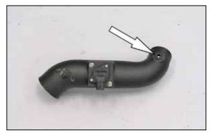
18. Install the mass air sensor assembly into the K&N<sup>®</sup> intake tube as shown and secure with the provided hardware. Install the crank case vent grommet into the K&N<sup>®</sup> intake tube as shown. NOTE: The arrow on the top of the sensor indicates the direction of air flow when the sensor is installed correctly.
