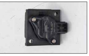
17. Install the mass air sensor into the  $K\&N^{\otimes}$  mass air adapter and secure with the provided hardware.
