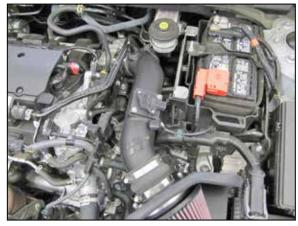
19. Install the K&N<sup>®</sup> intake tube into the coupling hoses, adjust for best fit and then secure with the provided hose clamps.
