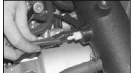
28. Remove the stock vacuum hose from the fuel pressure regulator, then install the provided silicone hose to the fuel pressure regulator and then onto the K&N intake tube as shown.
