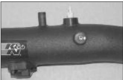
20. Install the provided 1/4" npt fitting into the K&N intake tube as shown.
