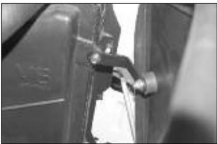
16. Secure the mounting bracket to the fan shroud with the original bolt.
