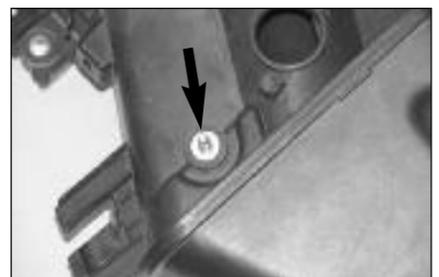
32. Using a pair of pliers, remove the engine cover mounting stud shown from the factory air box.
