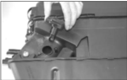
18. Remove the two screws that secure the mass air sensor to the air box assembly, then remove the mass air sensor as shown.
