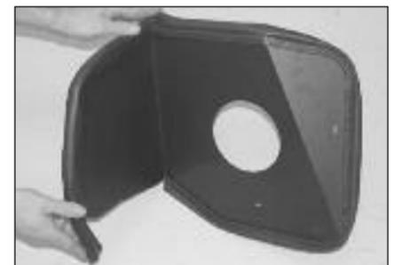
11. Install the provided edge trim onto the K&N intake tube as shown.
