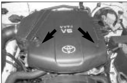
2. Loosen the two nuts that secure the engine cover, and then remove the engine cover from the engine.
