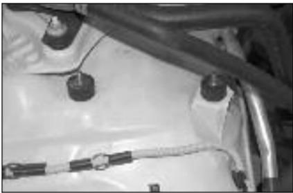
14. Install the two remaining rubber mounted studs to the original air box mounting holes as shown.
