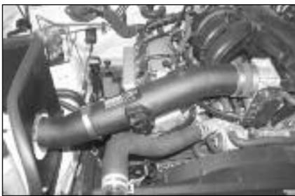
24. Install the K&N intake tube into the silicone hose at the throttle body and align with the bracket installed in step #23. Secure the intake tube with the hose clamps provided.
