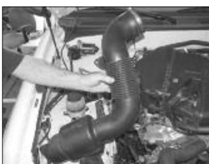
5. Remove the intake tube from the vehicle.
