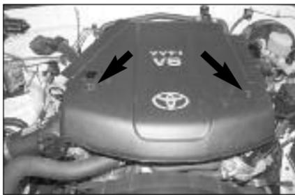
35. Install the engine cover and secure with the factory mounting nuts removed in step #2.
