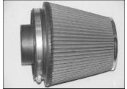
29. Install the filter adapter into the Filtercharger as shown.
