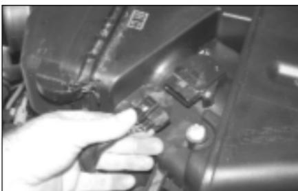
6. Disconnect the two mass air wire harness retaining clips from air box, then disconnect the mass air sensor electrical connection.
