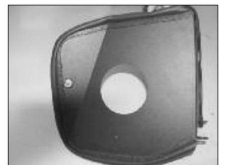
12. Install the rubber mounted stud to the heat shield with the provided hardware, but do not tighten completely at this time.
