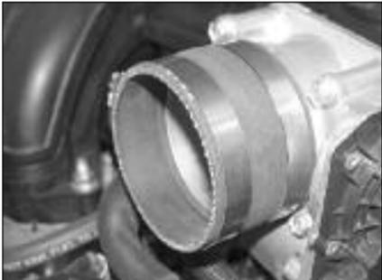
17. Install the silicone hose (08434) onto the throttle body and secure with the provided hose clamp as shown.
