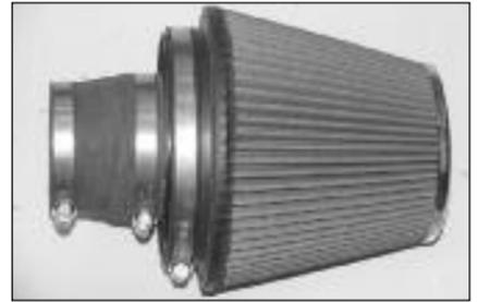
30. Install the silicone hose (08724) onto the Filtercharger assembly as shown and secure with the provided hose clamp.
