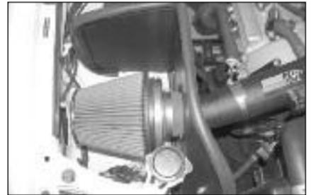
31. Install the Filtercharger assembly onto the K&N intake tube and secure with the provided hose clamp.
