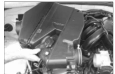
10. Remove air box assembly from engine as shown.
