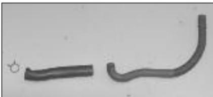
25. Remove the factory crank case vent hose from the valve cover and then remove the factory clamp and outer cover from the crank case vent hose as shown.
