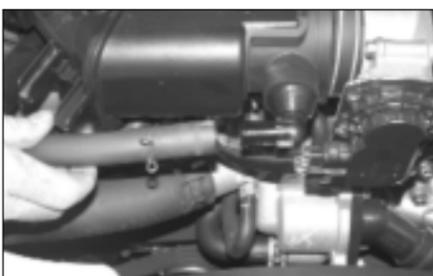
7. Remove crank case vent hose from air box as shown.
