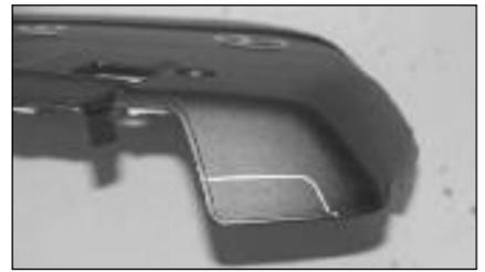
34. Using the provided template, mark the trim lines onto the engine cover and then cut with the appropriate tool.
