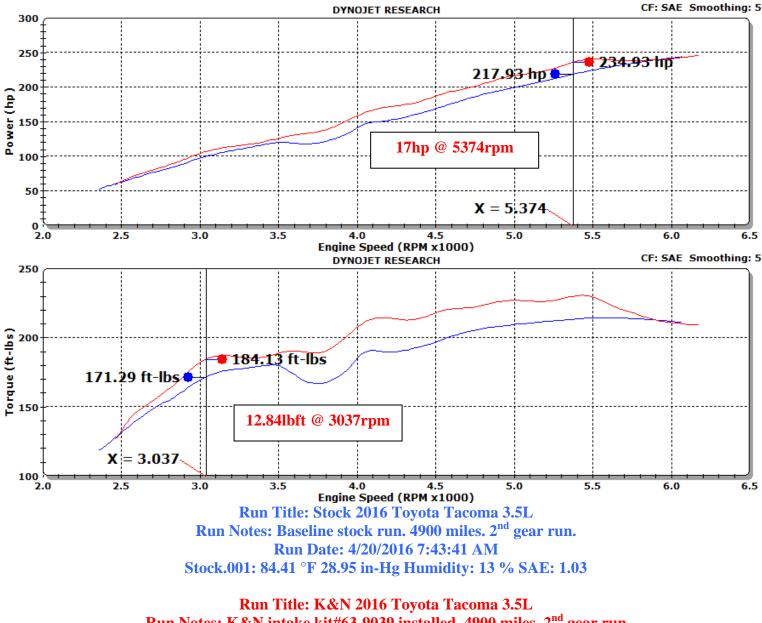
Run Notes: K&N intake kit#63-9039 installed. 4900 miles. 2<sup>nd</sup> gear run Run Date: 4/20/2016 9:46:53 AM K&N.002: 90.84 °F 28.96 in-Hg Humidity: 8 % SAE: 1.03
