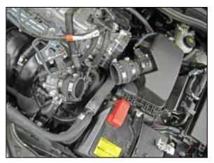
5. Install the provided hump couplers onto the throttle body and air filter housing and secure with the provided hose clamps.
