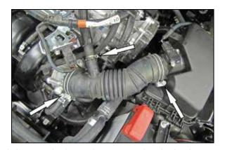
Loosen the hose clamps securing the intake tube and release the spring clamp on the crank case vent hose. Disconnect the crank case vent hose and then remove the factory intake tube from the vehicle.
