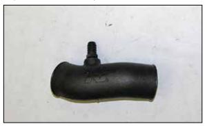
6. Install the provided crank case vent fitting into the K&N® intake tube as shown.
