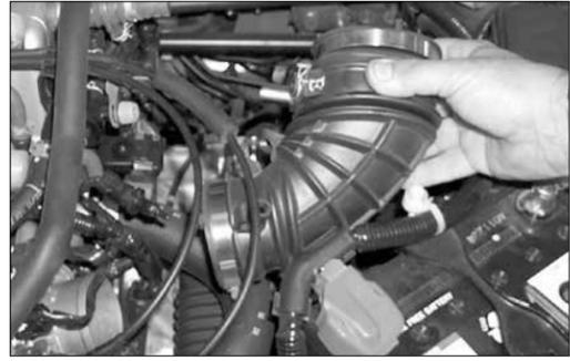
9. Loosen the hose clamp at the throttle body, then remove the stock intake tube as shown.
