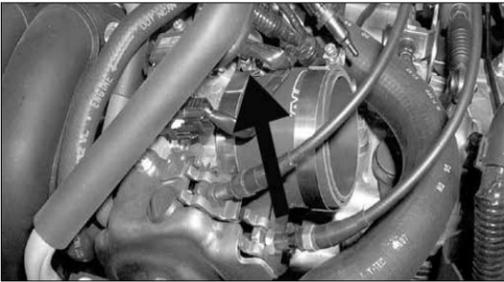
13. Install the silicone hose and hose clamps onto the throttle body and tighten as shown.
