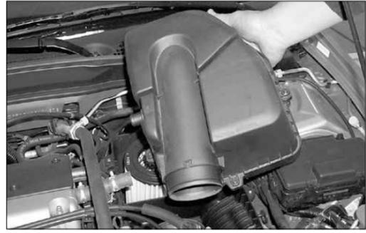
7. Loosen the five bolts that secure the upper air cleaner assembly, then remove the assembly as shown.
