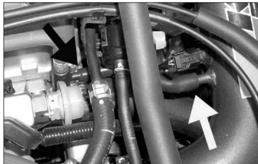
22. Connect the provided silicone hose to the IA bypass control thermal valve, then, connect the other end to the vent on the K&N intake tube as shown. Trim to fit if necessary. Supplied #004 hose clamp provided, can be used for improved seal.
