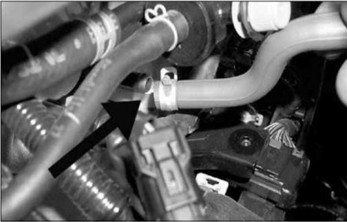
12. Remove the stock IA bypass control thermal valve vent hose as shown.
