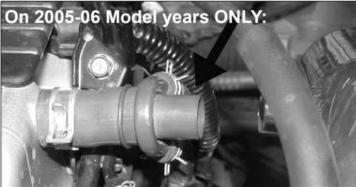
14. On '05-'06 models, remove the stock crank case vent hose as shown.
