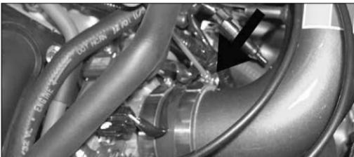
20. Tighten the hose clamp on the K&N intake tube as shown.
