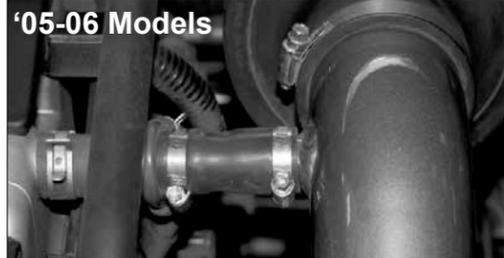
18. Connect the crank case vent hose to the vent on the K&N intake tube and slide the stock hose clamp onto the vent as shown. On 2005-06 model, use supplied hose and hose clamps and tighten.
