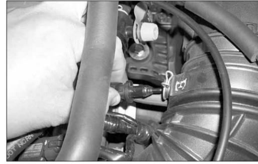
4. Depress the hose clamp at the air temperature sensor, then remove the air temperature sensor from the stock intake tube as shown.
