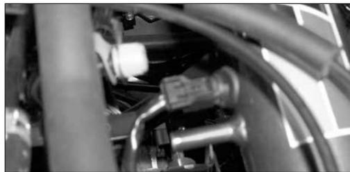
21. Push the air temperature sensor into the grommet in the K&N intake tube as shown.
