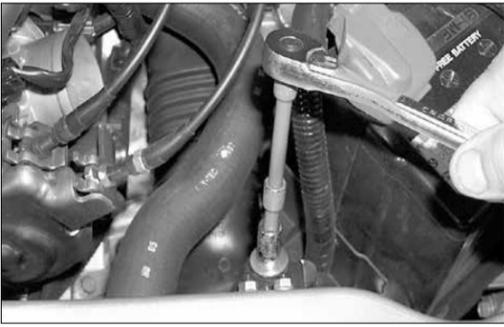
10. Loosen and remove the hex bolt that secures the air inlet duct as shown.
