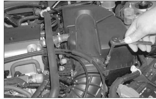
6. Loosen the hose clamp at the air cleaner assembly as shown.
