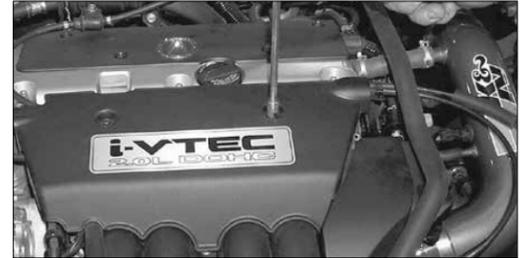
25. Reinstall the engine cover and secure with the original hex bolts as shown.
