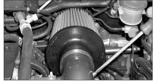
23. Install the K&N air filter onto the K&N intake tube, then, secure with the provided hose clamp as shown.
