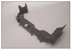
7. From underneath the vehicle, carefully remove the splash guard.
