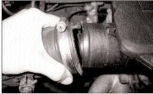
2. Unclip and remove the intake hose from the throttle body housing.
