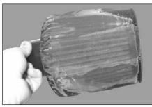
19. Install the K&N Drycharger onto the K&N Filtercharger as shown. NOTE: The Drycharger's water repellant properties will last up to two years. See parts list to re-order Drycharger if necessary.
