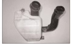
9. Unscrew the three bolts and remove the resonator box from the vehicle.
