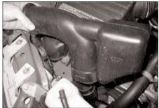
4. Carefully remove the intake snorkel from the vehicle as shown.
