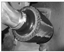
20. Fit the filter to the intake tube and secure the hose clamp supplied.
