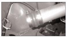
16. Fit the silicone hump hose to the intake tube using the #275 barrel clamp supplied. Make sure the tube is inserted about 1"/2.5 cm into the hose.
