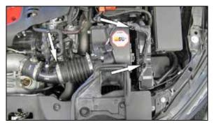
3. Release the upper air filter housing clips and loosen the hose clamp that secures the intake hose to the turbo inlet pipe. Remove the upper air filter housing and intake tube from the vehicle.
