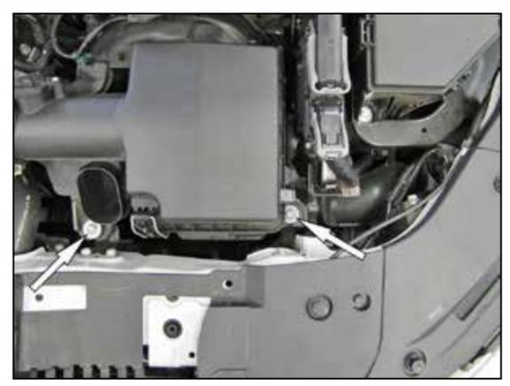
5. Remove the two bolts that secure the air filter housing and then lift up the intake assembly to remove it from the vehicle.
