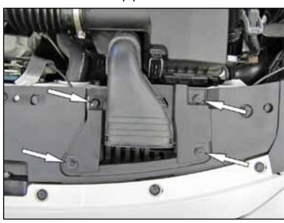
4. Remove the four pins that secure the fresh air intake to the core support. Remove the fresh air duct from the vehicle.
