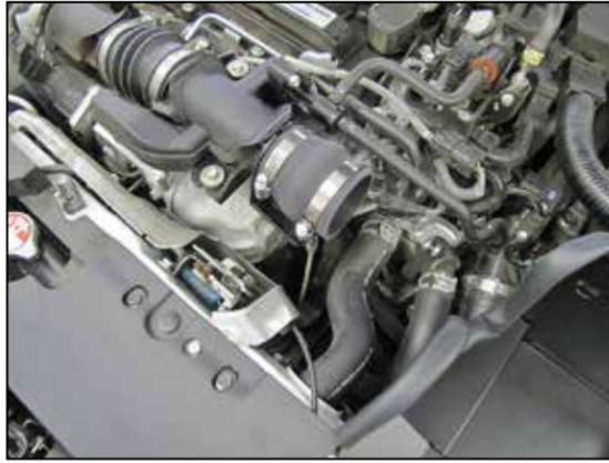
12. Install the provided hump coupler (08487) onto the turbo inlet and secure with the provided hose clamp.
