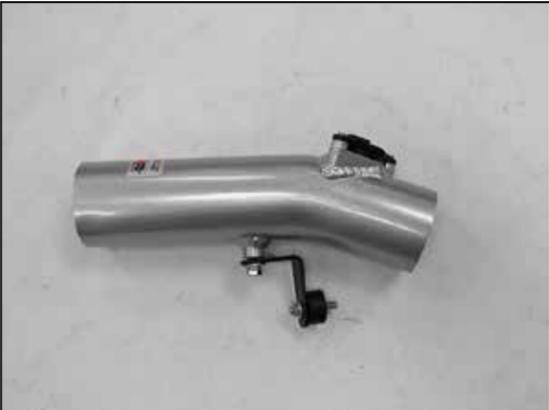
11. Install the mounting bracket assembly onto the K&N® intake tube as shown using the provided hardware.
