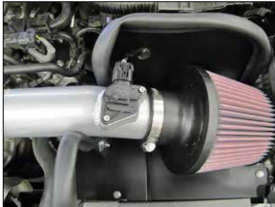
15. Route the mass air sensor wiring harness through the hole provided in the heat shield and then reconnect the mass air sensor electrical connection.
