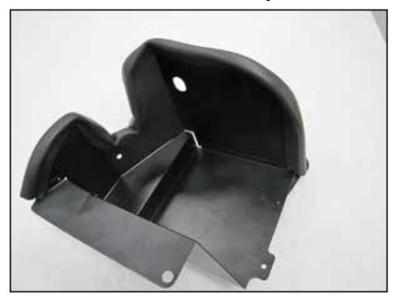
6. Install the provided edge trim onto the heat shield as shown, some trimming of the edge trim will be necessary.
