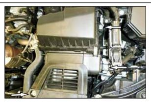
5. Remove the three bolts that secure the factory air filter housing and fresh air duct and then remove the assembly from the vehicle.
