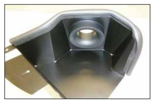
7. Install the filter adapter into the heat shield using the provided hardware and then install the edge trim onto the heat shield as shown.
