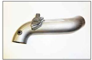
11. Remove the mass air sensor from the factory housing and then install it into the K&N intake tube using the factory screws. Install the provided PCV grommet into the K&N intake tube as shown.
