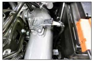
13. Reconnect the mass air sensor electrical connection.
