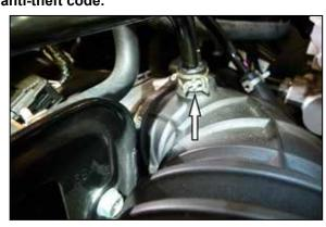
2. Release the spring clamp that secures the PCV pipe and then disconnect the pipe from the factory intake tube.
