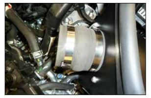
9. Install the hump coupler onto the filter adapter and secure with the provided hose clamp.
