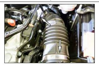
3. Loosen the hose clamps that secure the factory intake tube and then remove the tube from the vehicle.
