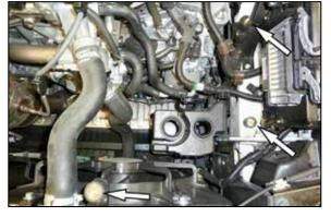
6. Install the three rubber mounted studs provided into the factory air box mounting locations.
