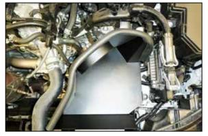
8. Install the heat shield onto the rubber mounted studs installed previously and secure with the provided hardware.
