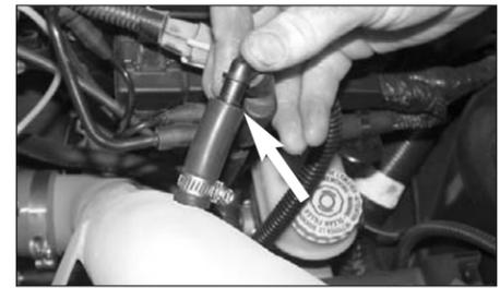
13. Reconnect the stock vent hose to the K&N Typhoon short ram tube as shown.
