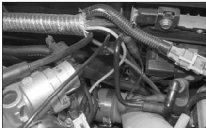
10. Tighten the hose clamp on the Typhoon intake tube as shown.
