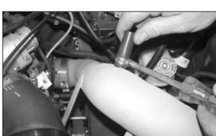
12. Slide the 2" silicone hose and hose clamp onto the vent on the K&N Typhoon short ram tube and tighten as shown.
