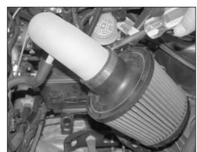
14. Install the K&N air filter onto the K&N Typhoon intake tube and secure with the provided hose clamp as shown.
