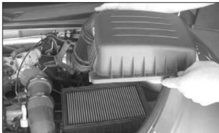
4. Unclip the upper air cleaner lid, then, remove the upper air cleaner assembly as shown.
