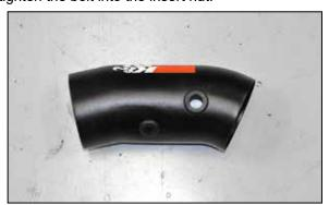
11. Install the two provided grommets into the  $K\&N^{\otimes}$  intake tube.
