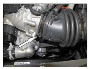
3. Loosen the hose clamp securing the intake tube to the throttle body.
