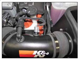
16. Reconnect the crank case vent hose and inlet air temperature sensor electrical connection.
