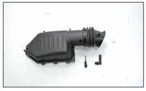
12. Remove the crank case vent and inlet air temperature sensor from the factory intake tube. NOTE: The inlet air temperature sensor is very fragile, use car while removing the sensor.
