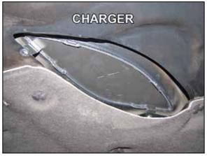
19. Install the guard so the mounting tabs are between the hood and the factory grid as shown.
