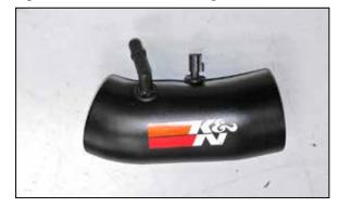
13. Install the crank case vent and inlet air temperature sensor into the K&N® intake tube. NOTE: the inlet air temperature sensor is very fragile, use care while installing the sensor.
