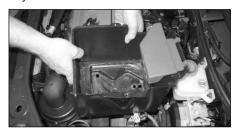
5. Carefully remove the battery tray from the
