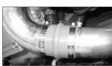
13. Install the second intake tube approximately 2.5cm / 1" into the hump hose.
