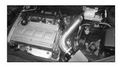
20. This K&N Typhoon intake kit has been designed to be used in two different configurations. In the case of inclement weather, the cold air tube can be removed and the filter can be clamped onto the first intake tube located in the engine compartment to avoid the possibility of ingesting water into the engine.
