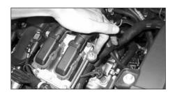
12. Fit the rubber vibration mount to the ECU housing.
