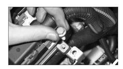
11. Unbolt and remove the bracket securing the two hose clamps from the ECU housing.
