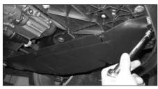
27. Re-install the left mud guard and the under tray to the car.
