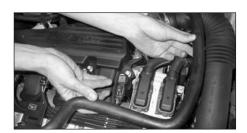
3. Unclip and remove the breather hose from engine and intake hose as shown.
