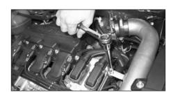
14. Mount the weld-on bracket of the A-tube to the rubber vibration mount using the nylock nut & washer supplied. Firmly tighten the nut.
