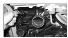
19. From the underside of the car, fit the silicone hump hose to the intake tube using the #275 barrel clamp supplied.
