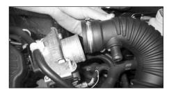
4. Unclip and remove the intake hose from the throttle body.
