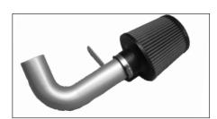
20. Fit the filter element onto the second intake tube using the #40 hose clamp supplied.
