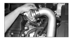
13. Fit the K&N Typhoon intake A-tube into the silicone hose, using the #275 barrel clamp. Do not yet tighten the #275 barrel clamp.
