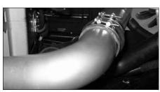
23. Fit the B-tube assembly into the silicone hump hose using the #275 barrel clamp supplied. Do not yet fully tighten the barrel clamp.
