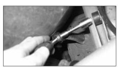
24. Fit the weld-on bracket on the B-tube onto the rubber mounting stud using the flat metal washer and nylock nut supplied as shown. Don't fully tighten yet!
