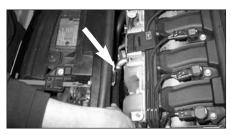
16. Fit the silicone breather hose onto the breather pipe on the oil filling pipe. For easier fitment, you may want to slightly grease the silicone hose and the pipe.
