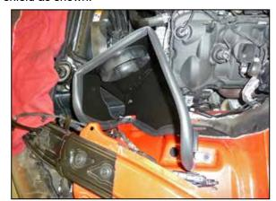
12. Install the heat shield assembly onto the inner fender and secure with the provided hardware.
