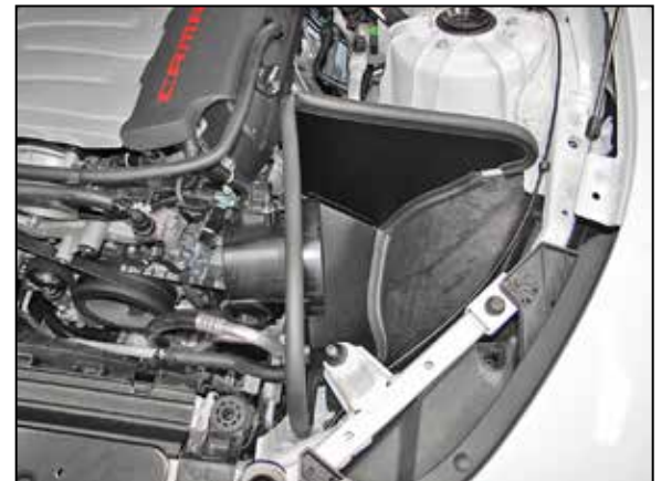
20. Install the K&N® heat shield assembly onto the air filter housing mounting grommets.
