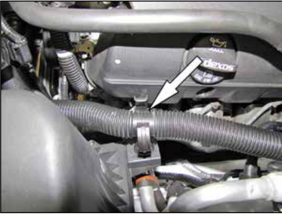
7. Open the clamp securing the sound tube to the air filter housing.
