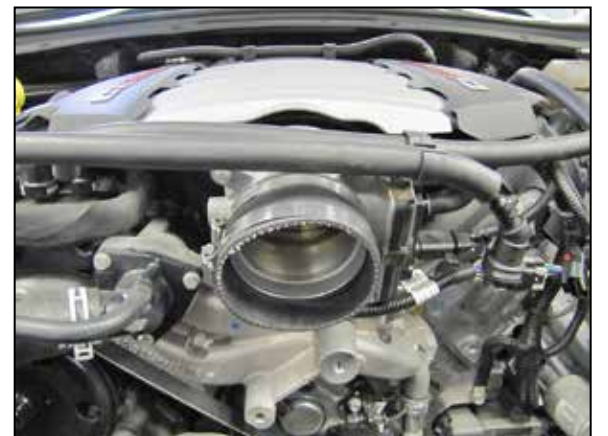
21. Install the provided coupler hose (08761) onto the throttle body and secure with the provided hose clamp.
