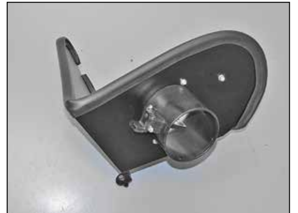
19. Install the mass air sensor into the K&N® mass air housing and secure with the provided hardware.
