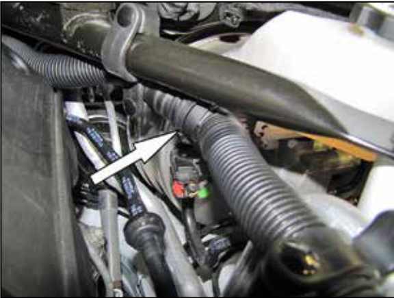
9. Disconnect the sound tube quick disconnect fitting and remove the complete sound tube system.
