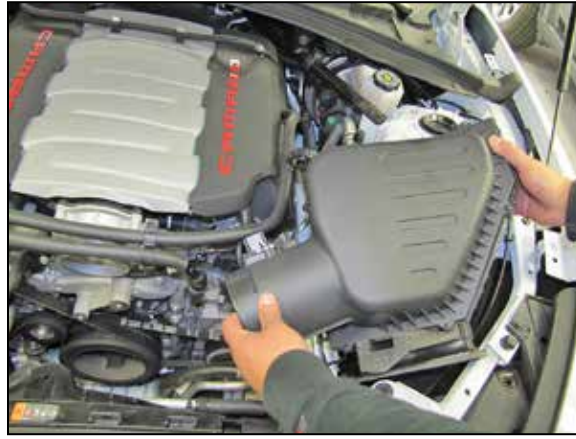
12. Lift up the air filter housing to dislodge it from the mounting grommets and then remove it from the vehicle.
