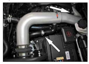
17. Connect the crank case vent hose to the 1/4npt fitting and secure with the provided hose clamp. Connect the factory air injection hose to the union installed into the 90° hose as shown.
