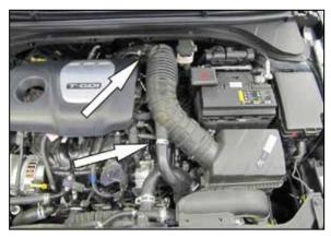
2. Release the spring hose clamps that secure the crank case vent hose and air injection hose to the factory intake tube and then disconnect the hoses from the factory intake tube.
