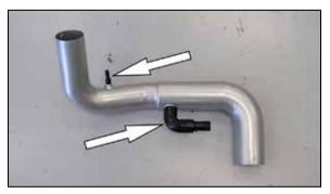
15. Install the crank case vent hose assembly and the 1/4npt vent fitting onto the K&N® intake tube as
