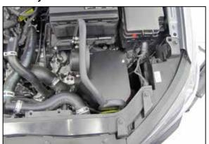
10. Install the heat shield into the vehicle and secure it to the rubber mounted stud and inner air filter housing mount with the provided hardware.
