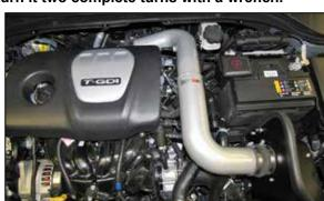
16. Install the K&N® intake tube assembly into the coupling hose at the turbo and then into the coupling hose at the filter adapter, adjust the tube for best fit and then secure with the provided hose
