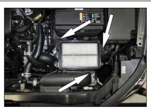
5. Remove the three bolts that secure the lower air filter housing to the inner fender and then remove the lower housing from the vehicle.
