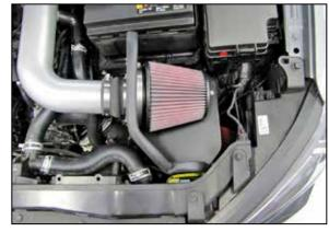
18. Install the K&N<sup>®</sup> air filter onto the filter adapter and secure with the provided hose clamp.
