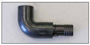
14. Install the provided union into the 90° portion of the cut crank case vent hose as shown.
