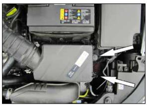
4. Release the two retaining clips that secures the air filter upper housing and then remove the intake tube and the air filter housing from the vehicle.
