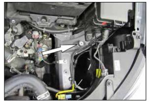
6. Install the provided rubber mounted stud into the air filter mounting location on the inner fender as shown.
