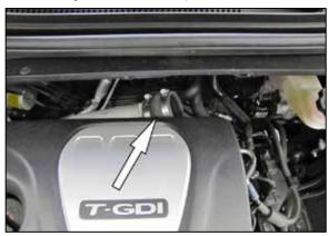
11. Install the provided coupler hose (08185) onto the turbo inlet and secure with the provided hose clamp.
