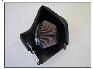
9. Install the provided edge trim onto the heat shield as shown, then install the K&N<sup>®</sup> air filter onto the filter adapter and secure with the provided hardware.
