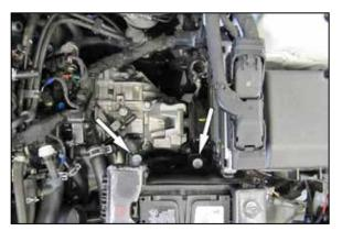
7. Install the two rubber mounted studs into the factory air filter housing mounting locations.
