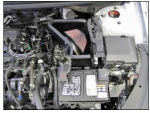
10. Install the heat shield assembly into the vehicle and secure to the rubber mounted studs with the provided hardware.
