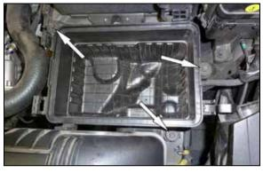
5. Remove the three bolts that secure the lower air filter housing and then remove the lower housing and fresh air duct from the vehicle.
