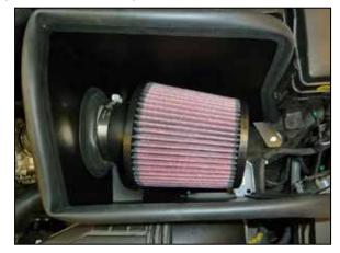
13. Install the K&N® air filter and secure with the provided hose clamp.
