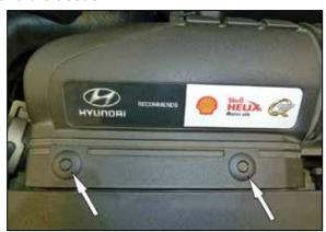
2. Push in the center of the retaining pins and then remove the pins from the fresh air intake duct.
