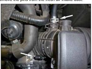
3. Loosen the hose clamp that secures the intake hose to the throttle body and then release the spring clamp that secures the PCV hose and disconnect the PCV hose from the intake tube.
