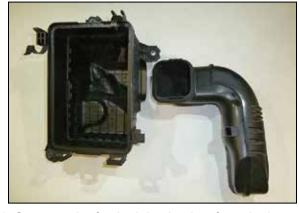
Separate the fresh air intake duct from the lower air filter housing.
