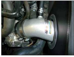
12. Install the K&N® intake tube into the heat shield and then into the coupler at the throttle body, align the tube for best fit and then secure with the provided hose clamp.
