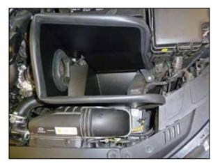
10. Install the K&N® heat shield and factory fresh air duct into the vehicle as an assembly. Secure the heat shield with the provided hardware and the fresh air duct with the factory pins.
