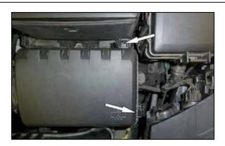
4. Release the two spring clips that retain the upper air filter housing, then remove the upper housing, intake tube and air filter from the vehicle.
