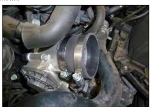
9. Install the provided coupler (084036) onto the throttle body and secure with the provided hose clamp.
