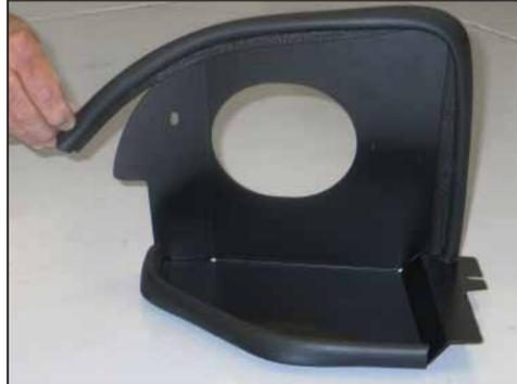
13. Install the long edge trim onto the heat shield as shown.
