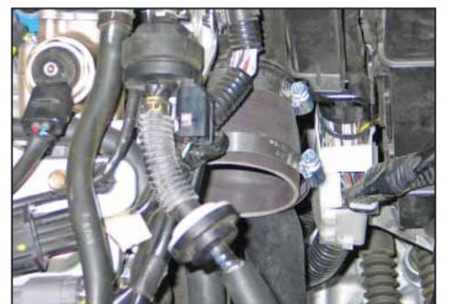
22. Install the provided silicone hose (#084016) onto the turbo inlet with the provided hose clamp as shown.
