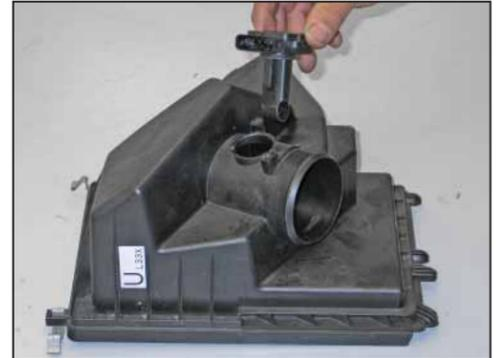
19. Remove the mass air sensor from the stock upper airbox housing as shown.
