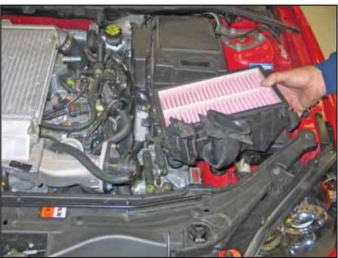
11. Lift upwards to dislodge the lower airbox from the mounting grommets. Remove the lower airbox from the vehicle as shown.
