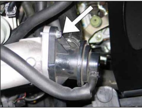
23. Remove the solenoid valve mounting bolt shown.
