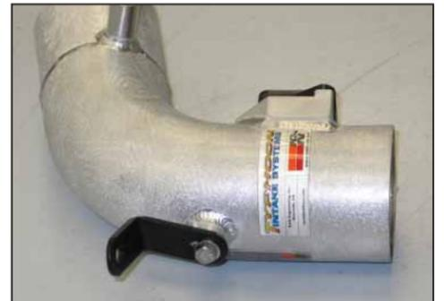
21. Install the tube mounting bracket (#07804) onto the K&N® intake tube with the provided hardware as shown.
