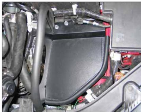
16. Install the heat shield onto the wiring loom mounting studs, then secure with the nuts removed in step #14.
