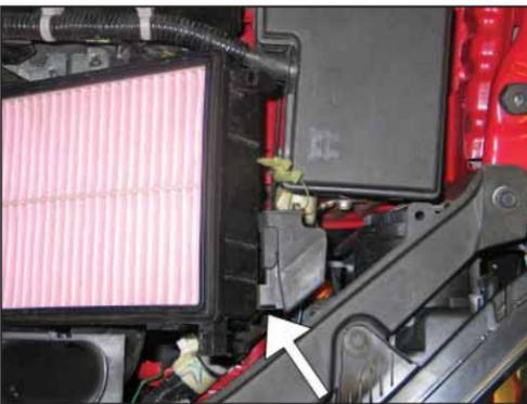
9. Remove the retaining clip, then slide the rubber airbox mount backwards as shown.
