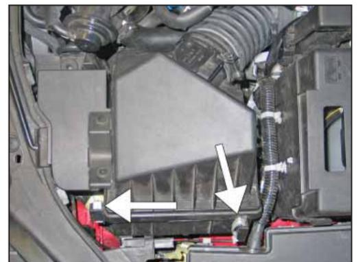
5. Release the two clips that secure the upper airbox housing to the lower airbox housing.
