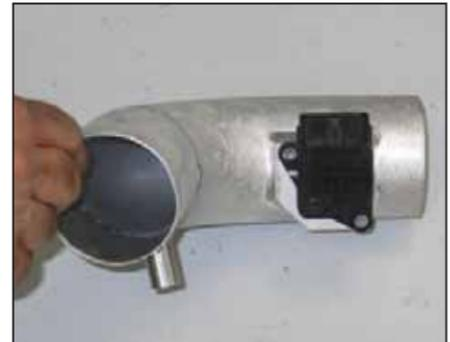
20. Install the mass air sensor into the K&N® intake tube with the provided hardware as shown.
