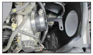
18. Install the provided coupling hose (08756) onto the throttle body and secure with the provided hose clamp.
