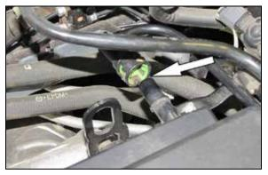
4. Release the green clip and then disconnect the crank case vent hose from the valve cover port.
