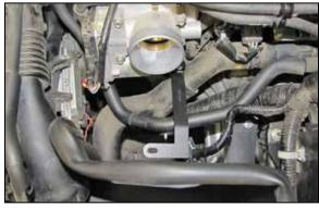
14. Install the tube mounting bracket onto the throttle body and secure with the factory bolt from the previous step.
