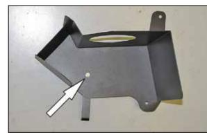
9. Install the provided bracket (083164) onto the heat shield using the provided hardware. NOTE: The bracket is to be fastened to the bottom side of the heat shield
