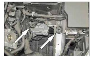
8. Remove the two air box mounting grommets shown. Install the provided rubber mounted stud onto inward air box mounting location. **NOTE: Be sure to use the two provided fender** washers and rubber washers. The fender washers go on either side of the factory bracket and the rubber washers go between the fender washers.
