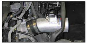
19. Install the K&N<sup>®</sup> intake tube assembly into the hose at the throttle body and align with the mounting bracket. Secure the tube with the hardware and hose clamp provided.
