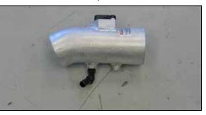
17. Install the 90° vent fitting into the K&N<sup>®</sup> intake tube as shown.
