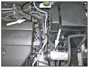
21. Connect the long end of the crank case vent hose to the fitting installed into the K&N<sup>®</sup> intake tube and then attach the open end to the valve cover port.
