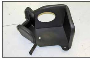
10. Install the provided edge trim onto the heat shield as shown. NOTE: Some trimming of the edge trim will be necessary.
