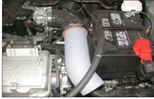
15. Install the Typhoon intake tube into the silicone hose as shown.
