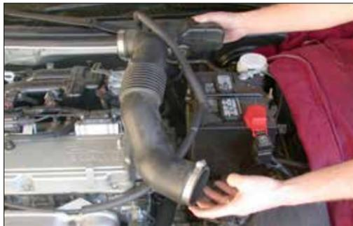
4. Loosen the hose clamps at the throttle body and at the mass air sensor, then, remove the stock intake tube as shown.
