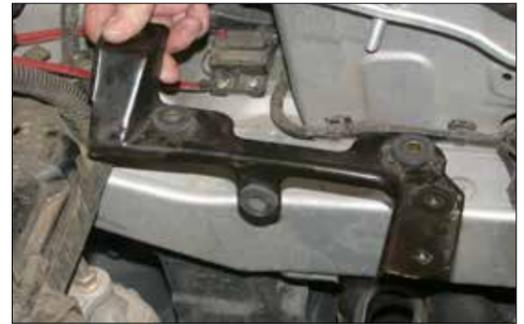
8. Loosen and remove the two bolts that secure the air cleaner support bracket, then, remove the air cleaner support bracket as shown.
