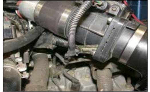
21. Re-clip the mass air sensor wire harness to the stock bracket on the mass air sensor as shown.
