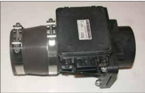
13. Install the silicone step hose and hose clamps onto the mass air sensor as shown.
