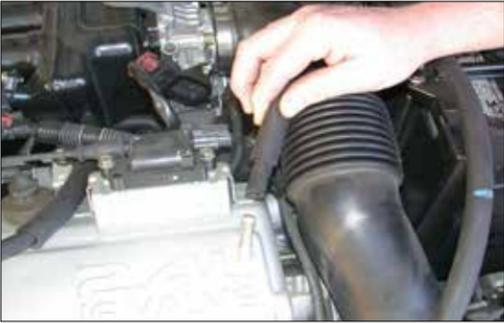
3. Disconnect the crank case vent hose from the cam cover as shown.
