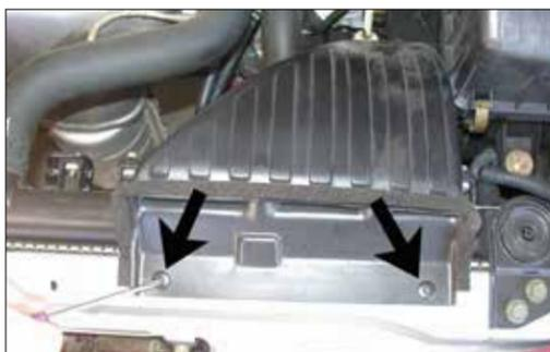
6. Depress the center pins on the air inlet duct as shown.
