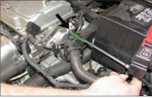
10. Remove the bolt that secures the wire harness to the engine as shown.
