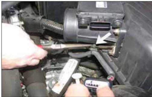
5. Unclip the mass air sensor wire harness from the air cleaner as shown.
