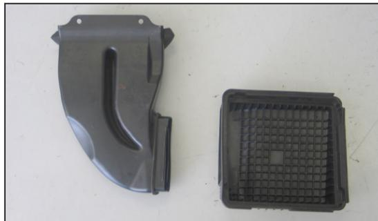
20. Remove the fresh air duct from the upper airbox housing.
