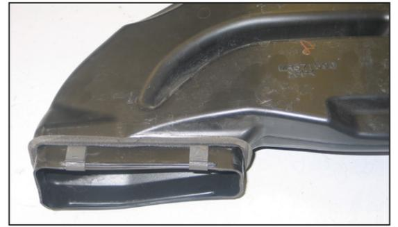
21. Install the two provided clips onto the fresh air supply duct as shown.
