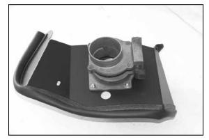
29. Install the MAF sensor onto the filter assembly as shown; secure with provided hardware.
