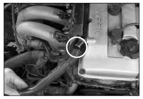
12. Using pliers, unclip the CVC hose and disconnect.
