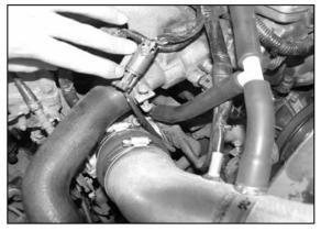
20. Install the 5-3/4" hose from the air bypass to the open port on the plastic "T".
