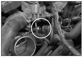
13. Remove the air bypass hose.
