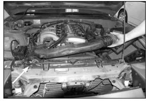
8. Remove factory air intake tube and upper air box. Disconnect the air resevoir hose.
