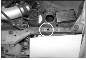
33. Remove the headlight bracket bolt.
