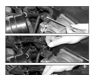
2. Loosen the hose clamp at the throttle body.
