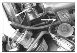
38. Install the 5/8"ID X 14" silicone hose from the open vent tube to the K&N $^{\circ}$  intake tube to the air bypass. Trim for best fit necessary.
