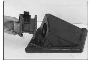
11. Remove the fresh air inlet tube by twisting and lifting upward.
