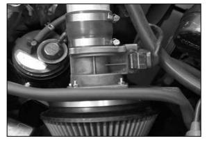
40. Reconnet the MAF sensor and reinstall the clip.
