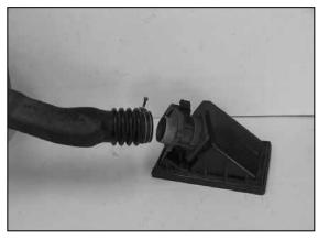
22. On the factory air intake tube, loosen the clamp to remove the factory air intake tube from the MAF sensor/air box assembly.
