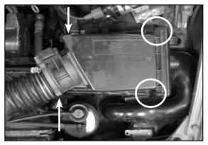
6. Unclip the 4 clips that secure the upper air box to the lower air box.
