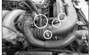
4. With pliers, squeeze hose clamps and disconnect the following hoses: cvc hose; air bypass hose; fresh air switching valve; and loosen the hose clamp on the air resevoir hose. Remove zip tie if present.
