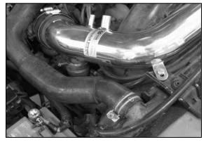
16. Install the K&N<sup>®</sup> intake tube, make sure that the air reservoir is connected at this time. Then install the provided bolt into the threaded hole on the original tube mounting point.
