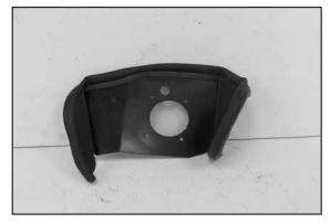
24. Install the provided edge trim onto the heat shield.
