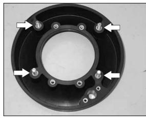
25. Install the studs onto the provided  $K\&N^{\otimes}$  filter adaptor.
