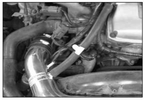
19. Install the 3-3/4" hose onto the intake tube and to the plastic "T'.
