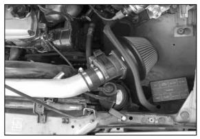
35. Install the filter assembly into the vehicle.
