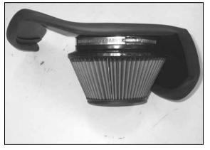
28. Install the heat shield onto the filter assembly as shown.
