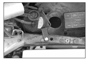
34. Install the spacer and bracket, then secure with provided hardware in the location where the bolt was removed in step #33.
