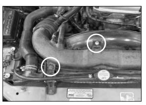
3. Remove the 2 bolts that secure the factory air intake.
