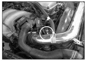
21. Reinstall the fresh air switching valve hose to the intake tube. Reattach any loose zip ties that were loosened.
