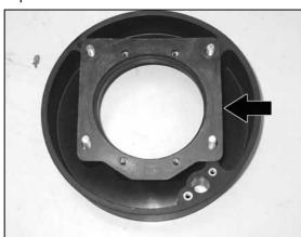
26. Install the gasket onto the K&N $^{\mbox{\tiny \$}}$  filter adaptor as shown.
