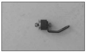
31. Stack washers around the "C" bracket and secure with rubber mounted stud (Do not tighten completely).
