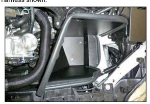
12. Install the heat shield into the vehicle so the mounting studs insert into the factory mounting grommets then secure the heat shield and wiring harness with the hardware provided.
