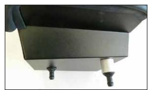
10. Install the heat shield mounting studs as shown using the provided hardware and spacer.
