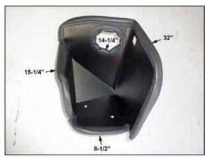
9. Install the edge trim onto the heat shield as shown.
