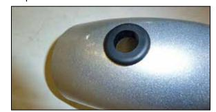
14. Install the provided grommet into the K&N® intake tube.
