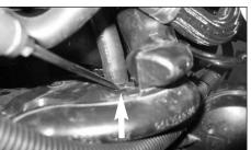
14. Carefully unclip and remove the air pump hose from the resonator box as shown.
