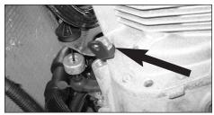
21. Remove the indicated nut from the gear box housing. Fit the bracket supplied onto the gear box housing using the original nut.
