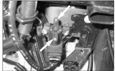
10. Fit two rubber tips supplied onto the electronic vacuum switch from step 7 as shown.
