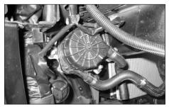
20. Re-install the air pump using the original hardware as shown.
