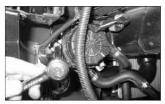
17. Remove the bolts securing the air pump to the vehicle, so that the air pump can be moved out of the way.
