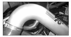
32. Fit the breather hose onto the vent on the K&N Typhoon intake tube as shown. Re-install the battery air breather tube which was removed in step 6 to the vehicle.
