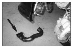
19. Unclip and remove the cold air intake tube from the vehicle.
