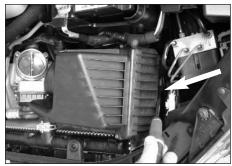
3. Unclip the air box from the air box support bracket as shown.
