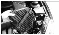
4. Carefully remove the complete air box assembly from the vehicle.
