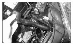
6. Remove the battery air breather tube from the vehicle.
