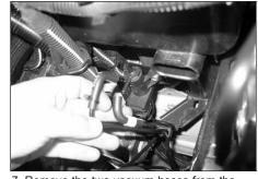
7. Remove the two vacuum hoses from the electronic vacuum switch as shown.
