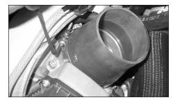
25. Fit the silicone stepped hose onto the throttle body using the #48 hose clamp supplied.
