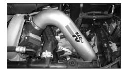
33. Align the intake tube for best fit and clearance, then, firmly tighten the hose clamp and M6 bolt and M6 nut. To provide more clearance between the filter and the arch liner you can insert the tube further into the silicone hose of the throttle body.
