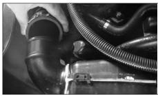
13. Unclip the intake snorkel from the resonator box.
